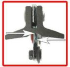
If the breaker is too loose you can tighten the rivet by placing the head of the rivet on a solid surface and hitting the open side of the rivet with a ball peined hammer to squeeze the aluminum to the metal handles. If you are only using it for thin glass all the time you can superglue the aluminum breaker so it stays in that position permanently.
