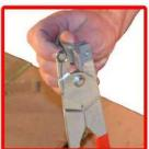
First stand the cutter up with the handles touching the bench, grab the aluminum breaker head between your pointing finger and thumb of each hand as in the pictures, then roll the breaker down and forward so it will swivel on the rivet thus closing the gap and allowing us to cut and squeeze some ridiculously narrow and thin pieces, if it is stiff to move you can place one side of the breaker in an open vice and then just push the handles in either direction.
